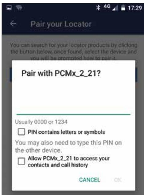
Select the device name. A prompt for the pairing code will appear. Insert 1234 and press OK. The device name will now appear under Paired Devices.
