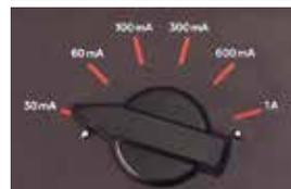
When the transmitter is operating, the selected current will remain at a constant level, unless the input power supply limit is reached.
