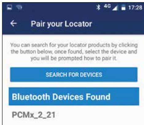
Press **SEARCH FOR DEVICES**. On the PCMx receiver press the  $\text{f}$  key to initiate pairing. The name of the device will appear underneath **BLUETOOTH DEVICES FOUND**.
