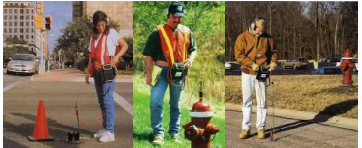
Downtown leak survey on main line valve
