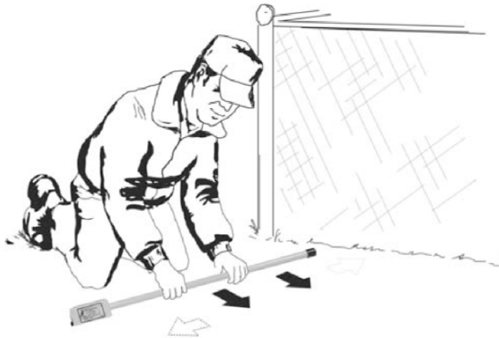
Figure 13: Searching in the Vicinity of a Chain Link Fence
