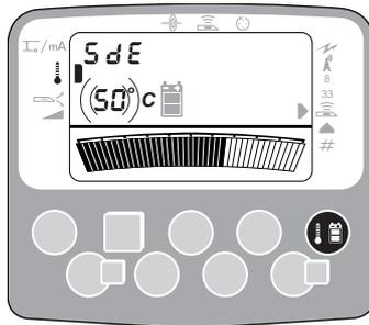
At 80°C (170°F) the bore must be halted to allow the sonde to cool or damage may occur. The Sonde stops transmitting Roll/Tilt information until it has cooled to 50°C.
