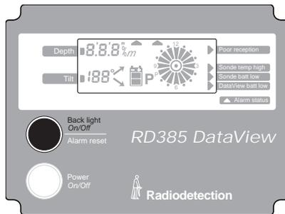
The DataView display will mimic the Receiver display while the data is being received with good signal strength.
