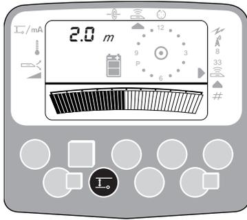
Press the Depth key to calibrate. The Receiver will display the calculated depth, beep twice and return to the DataSonde mode.
