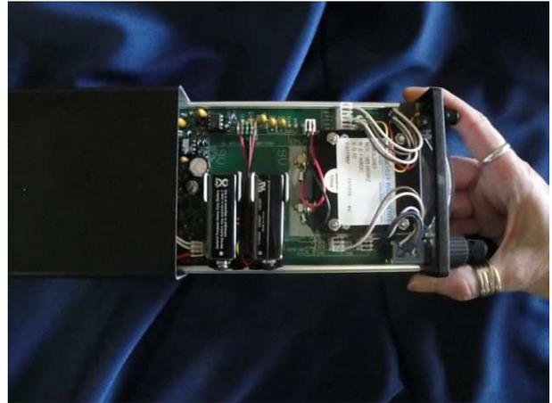
To replace the batteries, remove the two screws from the back plate. To access the batteries slide the top Black cover on the S30 back away from the removed screws. The batteries are immediately accessible and removable, replace batteries and replace black cover and screws.
